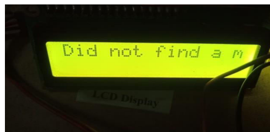
Fig 5: If a person who is not enrolled tries to vote/ uses his vote the lcd displays did not find am and buzzer sound will be generated.
